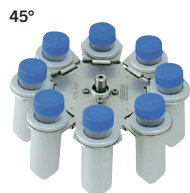
Swing-out rotor, 8-place, n= 5,000 min -1 , RCF 3,857, for 8 x 50/15 ml, stainless steel, with suspensions, aluminium.
