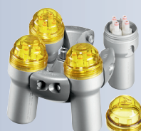
Swing-out rotor 01324, 4-place, illustrated with carrier 01490 and lids 01492 n = 4,500 min -1 , max. RCF 3,328 for max. 4 x 100 ml
